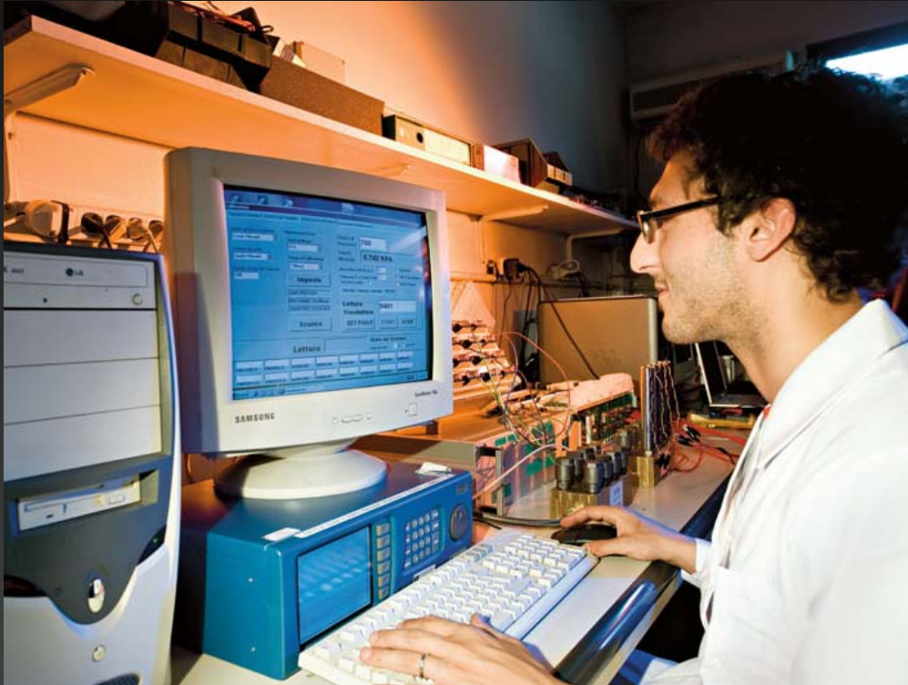
Pressure transducer calibration desk
