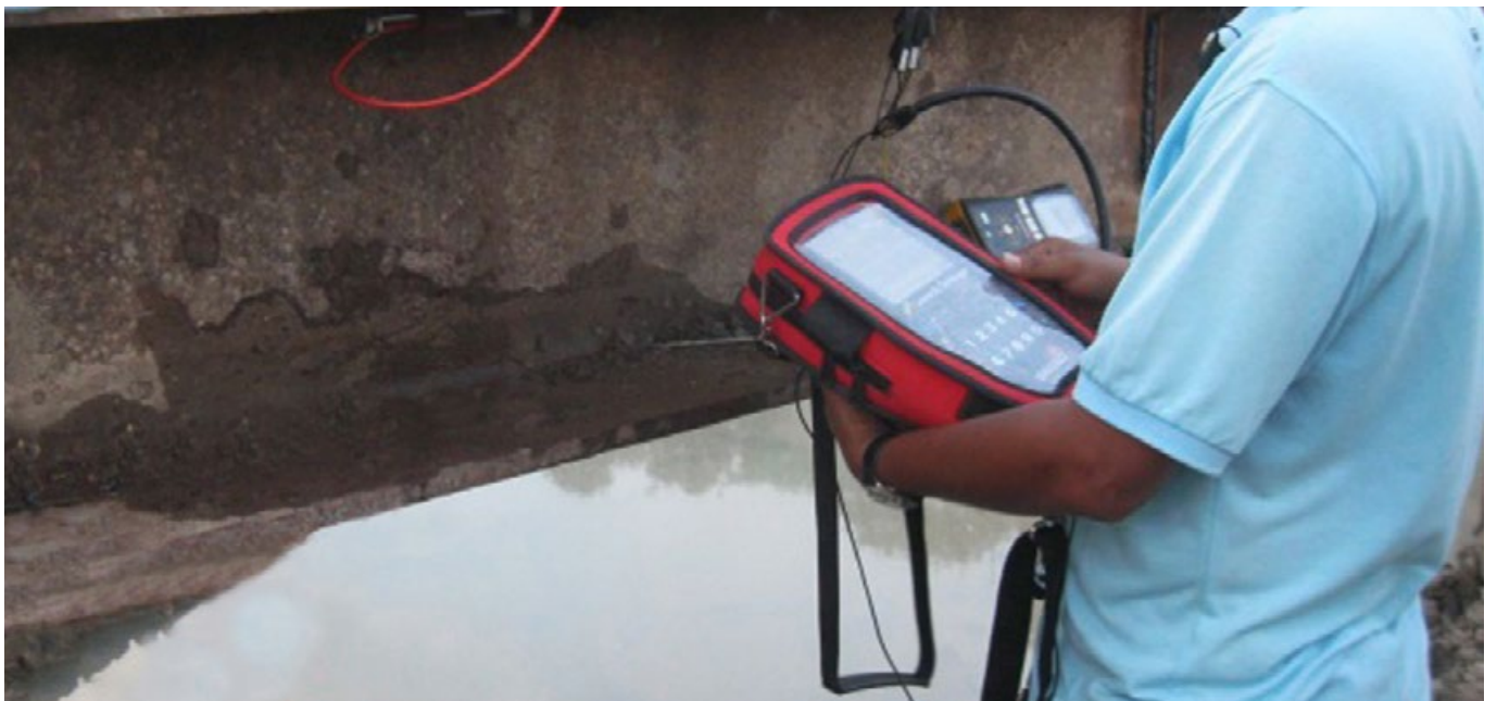
Anchor tensioning with the installed anchor load cell
