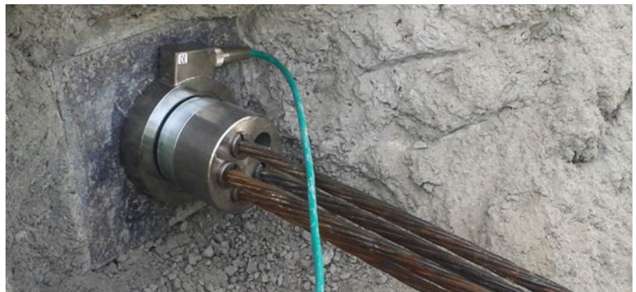
Sisgeo's anchor load cell
